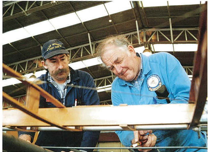
Busy in the workshop are volunteers Colin Stacey and Peter Tyers. They are working on the uncovered wing of the museum's airworthy Sopwith Pup replica Photograph by Teena Cardillo
